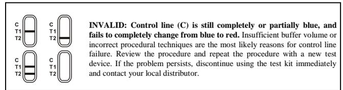
**INVALID: Control line (C) is still completely or partially blue, and fails to completely change from blue to red.** Insufficient buffer volume or incorrect procedural techniques are the most likely reasons for control line failure. Review the procedure and repeat the procedure with a new test device. If the problem persists, discontinue using the test kit immediately and contact your local distributor.
